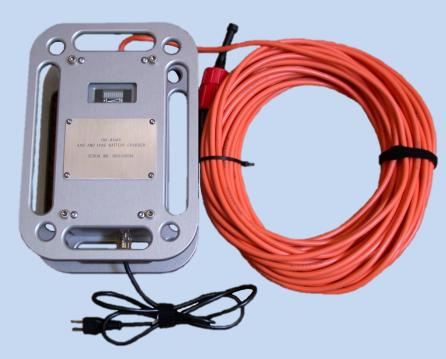
The Battery Charger was designed to be used on the deck of the ship; leaving the more valuable Programming Unit on deck for long periods during charging, is undesirable.
